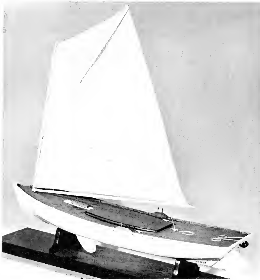
EGG HARBOR MELON-SLED GUNNING SKIFF from lower Barnegat Bay, New Jersey. Rigged model USNM 25658 showing a typical boat of this type. (Smithsonian photo 44697-a.)
